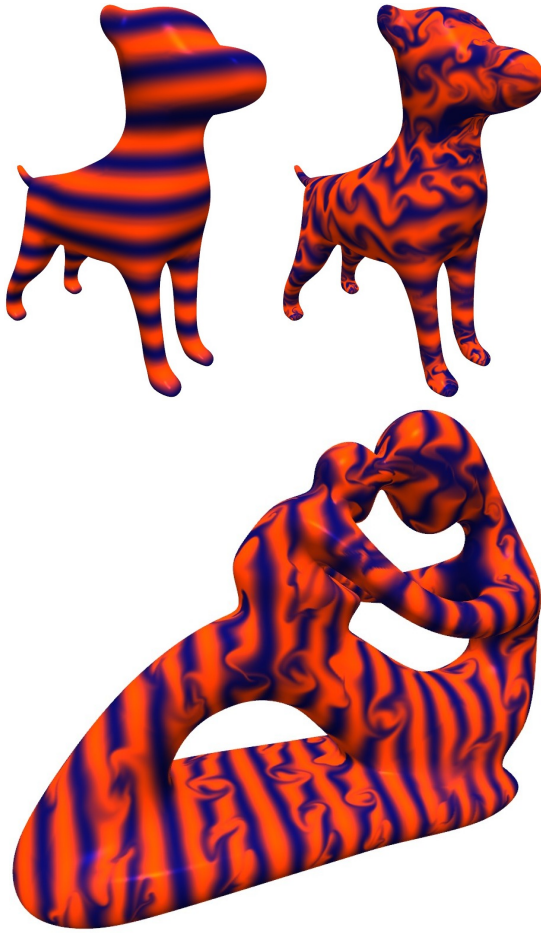
Fig. 6. Forces following circular paths on the dog and fertility models.
